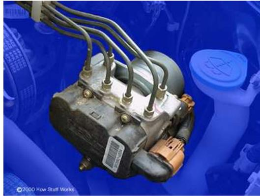
**Anti-lock brake pump and valves**
